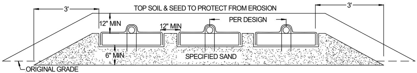
FIGURE 12: SECTION VIEW – SLOPED RAISED EDA SYSTEM
