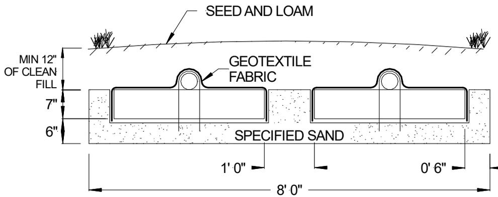
FIGURE 10: SECTION VIEW – SLOPING BED SYSTEM
