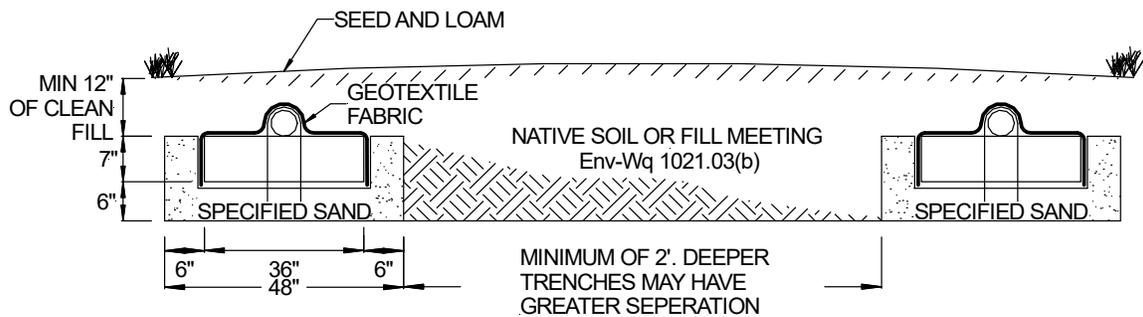
FIGURE 7: SECTION VIEW – TRENCH SYSTEM – SLOPING SITE
